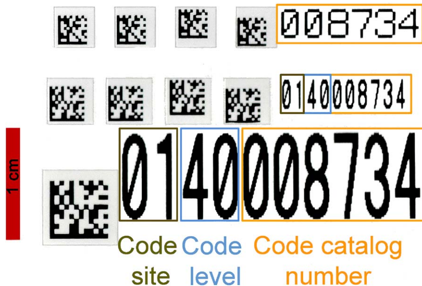
Fig. 1. Label with DM code: top row 2.5 × 2.5 mm DM code capable of storing the catalogue number code; middle row 3 × 3 mm DM code that contains the level and catalogue number codes; bottom row 5 × 5 mm DM code with the series of codes – site, level and catalogue number.
