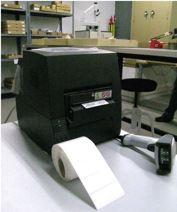
Fig. 3. Accessories used to apply the DM code: (a) desktop digital thermal wax printer (real size 240 × 200 × 200 mm); (b) laser reader for reading two-dimensional codes.
